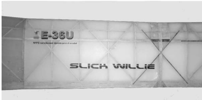
Fig. 8 Union Jack geodetic rib construction in the Slick Willie's wing
